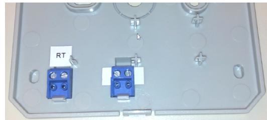
To make the extra inputs available an extra connector needs to be put into the thermostats back.
