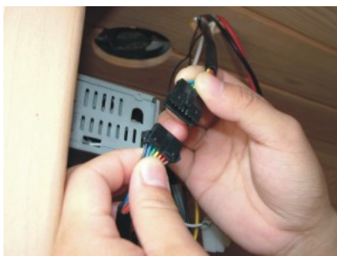
FIG-20 Link the control panel connectors
