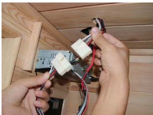
FIG-18 Link the CD connectors
