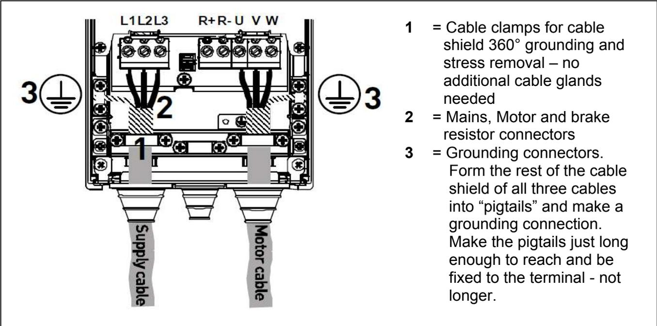
Fig. 5. SmartDrive HVAC power connections
